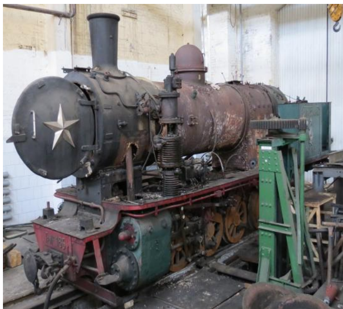
The 750mm gauge Gr-185 0-8-0 from the Rostov children's railway under repair at Tikhoretzkaya, stripped down and awaiting a new boiler. Photo by Vladimir Burakov.
